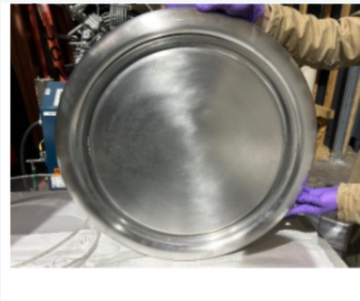
Cleaned HV electrode being prepared for magnetic screening.
