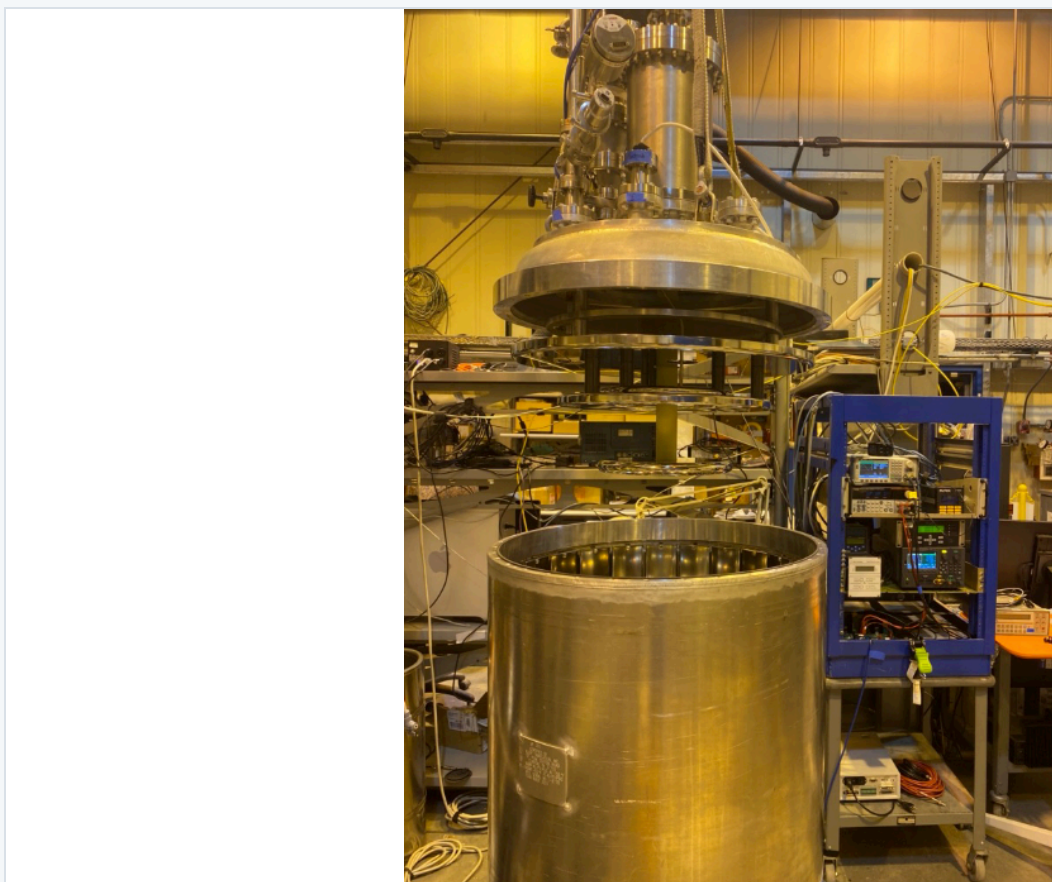
Central assembly and dewar during integration. I supported the installation and connected the surrounding cryogenic, vacuum and instrumentation systems.
